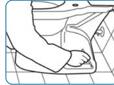
4. The floor is marked through the temporarily mounted WC mounting holes.
