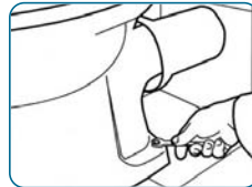
6. The WC is mounted on the stop in the floor and the waste water pipe and fastened to the floor.
