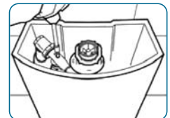
12. The cistern water level is set.
