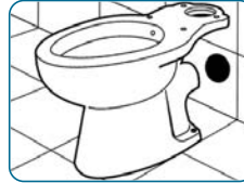
1. The waste water outlet is prepared to match WC outlet size.
