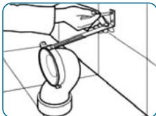
1. S' bend is mounted in place and fastened to the wall with a metal sheet.
