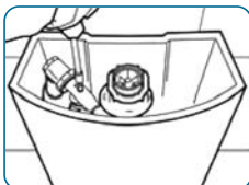
7. The spiral pipe is mounted on the cistern water inlet.
