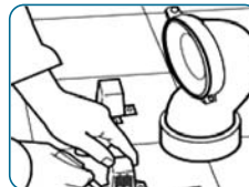
4. The WC is removed and plastic mounting element is placed on the floor so as to centre the hole axis.
