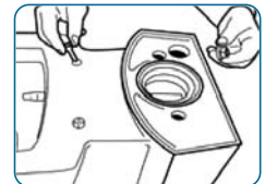
6. The cistern and WC seat and cover are mounted and water leak test is made.
