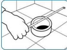
1. Waste water outlet centre is adjusted relative to the waste water pipe.
