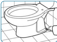
6. The WC is put in place and mounted properly.
