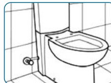
10. The cistern clean water inlet is attached to the tap.
